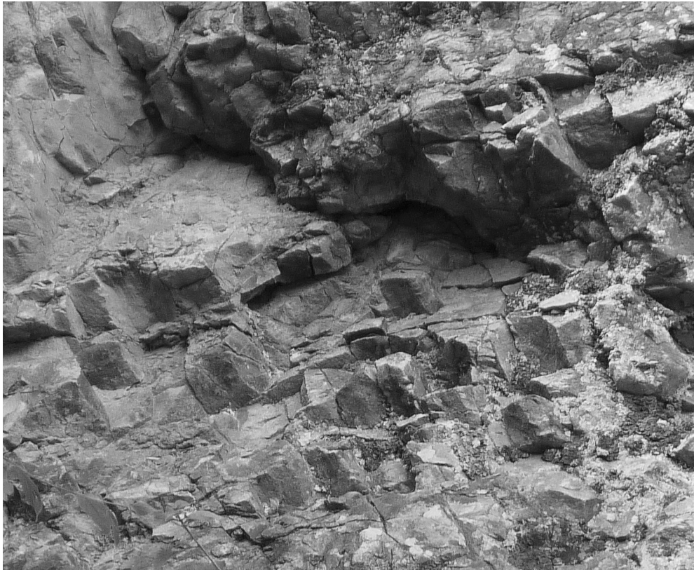
Fig. 4. Range of RQD values interpreted by independent professionals at three rock exposures in Sydney. obs., observations.
